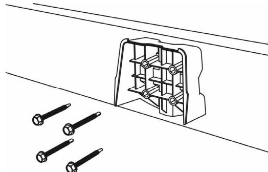
To mount the bracket on a flat vertical surface, or a round wooden post, use the 4 x tek screws included with the unit.
